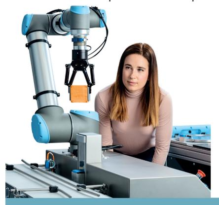
Pick & place operations are one of the automated tasks for which cobots from Universal Robots are most often used. Our cobots are ideal for a wide spectrum of such setups, from those requiring high positioning accuracy to those requiring a vision system to locate the part. The high repeatability provided by UR cobots ensures exceptional accuracy in all kinds of automated pick & place taskings.
